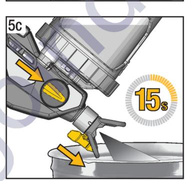
Note: Store Sprayer filled with Pump Armor™ (included) storage fluid for trouble-free startup.
