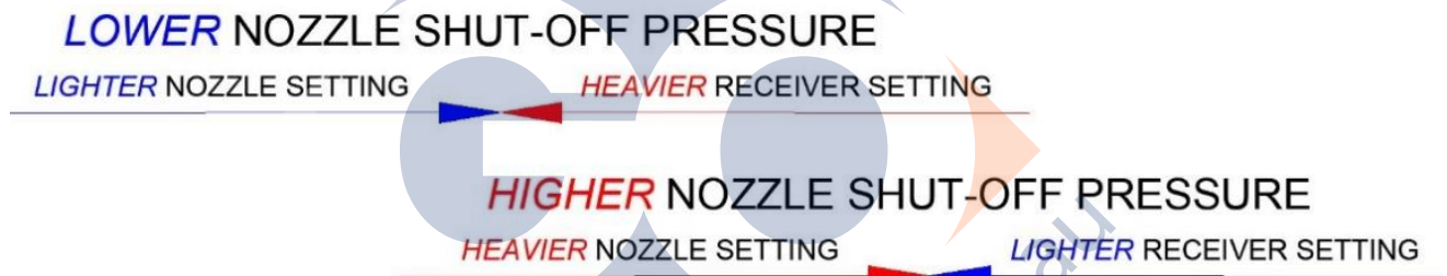
Figure 10 - Relationship Between Nozzle and Receiver Spring Settings
