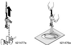
When finished with stencil, wrap hose around top of hopper and attach material dispenser to vertical arm mount.
