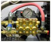
4 pole motor Pressure gauge Brass unloader Thermal dump Brass strainer Bertolini pump
