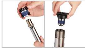
1) Insert pre-oiled packing cartridge assembly
