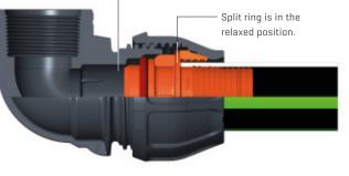
Insert fully installed into the pipe up to the shoulder of the insert.
