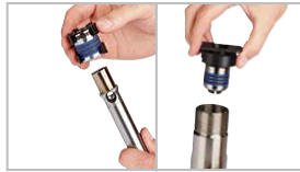
1) Insert pre-oiled packing cartridge assembly
