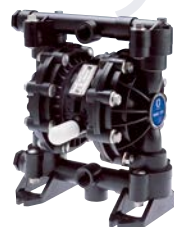
Husky 515 1/2 in (12.7 mm) connection Max flow: 15 gpm (57 lpm) Polypropylene, acetal, PVDF
