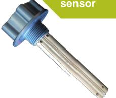
The Model T/LL350 series is a range of highly advanced sensors for continuously measuring the contents of a fuel tank. The unique feature of the T/LL350 is that it recalibrates itself when a liquid with a different dielectric constant is used. For example, if it is used in a tank of conventional diesel, then the user can refill with bio-diesel and the sensor will correct the output level automatically.
