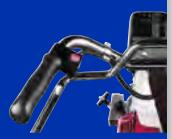
Electric Gun Control—Manual or automatic paint and bead guns with a push of a red button.
