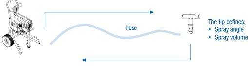
The tip size tells the pump how hard it must work.
