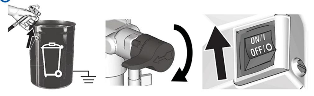
When paint comes out of the gun, release trigger. Turn gun trigger lock to locked position. Thread spray tip and guard assembly to gun.
