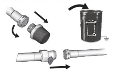
TO SAVE PAINT IN HOSE: Trigger gun into paint pail, turn Prime/Spray Valve forward to SPRAY and turn Power Switch ON. When water comes out of gun, keep gun triggered and aim into waste pail. Continue to flush until water runs clear.
