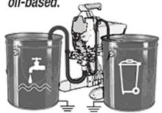
With the Prime/Spray Valve down to **PRIME**, press PushPrime™ button twice, turn Pressure Control Knob to Prime/Clean setting. Turn Power Switch **ON**.
