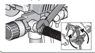
2 Turn gun trigger lock to locked position. Unthread spray tip and guard assembly.
