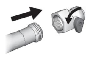
Unscrew inlet strainer from suction tube and place in waste pail for cleaning. Thread Power Flush attachment to suction tube. Turn Power Switch ON and let water run through drain tube for 20 seconds. Turn Power Switch OFF.
