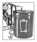
Submerge suction tube in water if spraying water-based material or flushing fluid if spraying oil-based.
