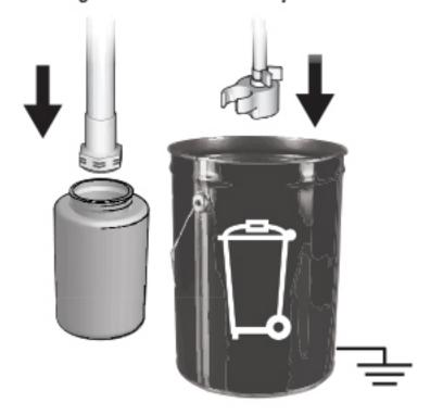
Turn Prime/Spray Valve down to **PRIME**. Turn Power Switch **ON**. Turn Pressure Control Knob to Prime/Clean setting.
