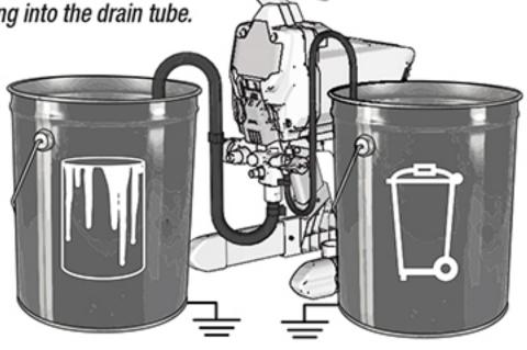
Trigger gun into waste pail, turn Prime/Spray Valve forward to SPRAY and turn Power Switch ON.
