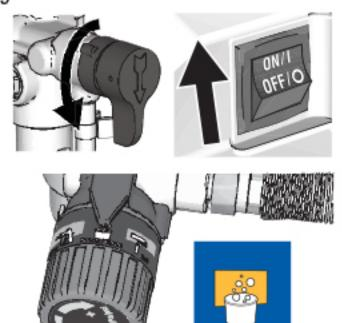
When Pump Armor comes out of drain tube, turn Pressure Control Knob to lowest setting and Power Switch **OFF**.
