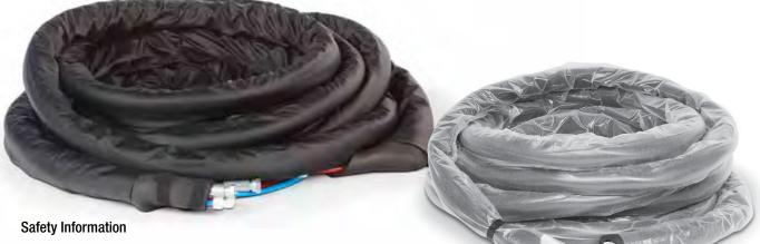
Remember to check your airless hose for kinks anywhere along its length. The hose should also be closely examined for splits, cracks or abrasions. Bulging anywhere on the hose or any amount of separation from the coupling could lead to hose failure and it should be replaced. For optimum hose life, never exceed the hose's rating for pressure and temperature.
