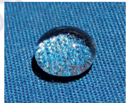
Known as the 'Lotus effect' treated fabric repels water
