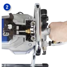
Remove pump section
