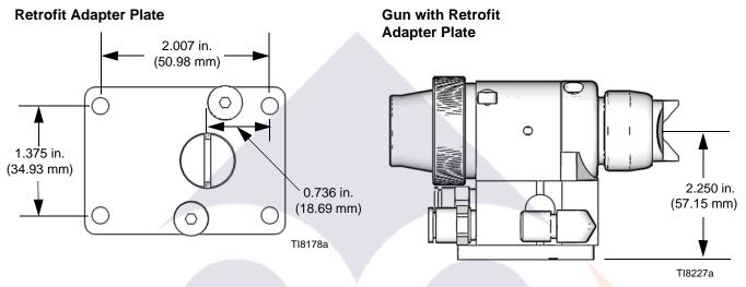
Fig. 26: Mounting Hole Layouts
