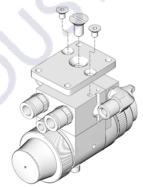
Fig. 5: Retrofit Adapter Plate
