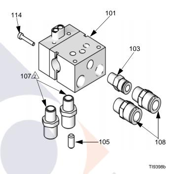
Fig. 20: Manifold with Bottom Fluid Ports
