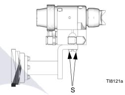
Fig. 4: Stationary Support Mount
