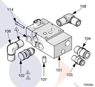
Fig. 21: Side Fluid Ports and Fan Adjustment Valve
