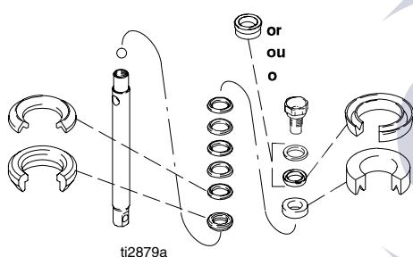
Soak leather packings in SAE 30W oil for 1 hour before assembly.
