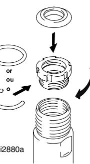
Loosely install packing nut onto cylinder.
