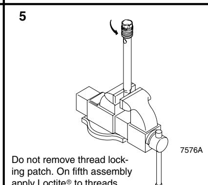
Do not remove thread locking patch. On fifth assembly apply Loctite® to threads.
