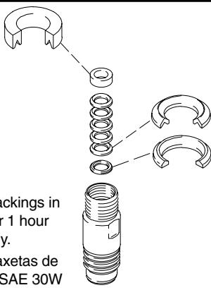
Soak leather packings in SAE 30W oil for 1 hour before assembly.
