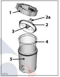
4. Return excess fluid to original container. Hold the FlexLiner (4) in place when pouring.
