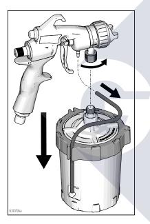
Loosen ring (1) from cup (5). Remove ring (1) and cover (2) from cup. Verify FlexLiner remains in cup upon removal of cover and ring.
