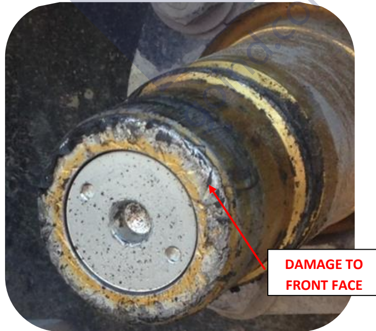
Figure 20 - Wear to Front of a non-Banlaw Aluminium Receiver
