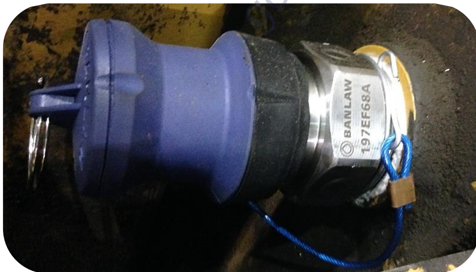
Figure 16 - Banlaw Receiver Installed with Dust Cap
