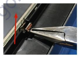
3. Press in one of the side tabs on the display until it is disengaged, and then press in the other side tab. Flip the LCD display down when both side tabs are disengaged.
