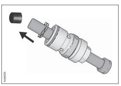
2. While holding the pump body upside down start threading the new packing assembly in by hand.
