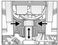
b. Push on pump rod to slide pump assembly back on to mounting pins.
