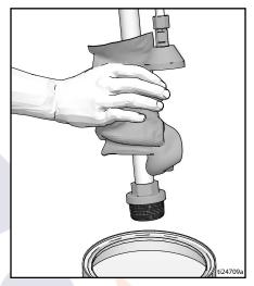
4. Place fluid intake in flushing fluid. Use water for water-based paint and mineral spirits for oil-based paint. Place drain tube in waste pail.
