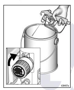
7. Stop triggering gun. Move gun to waste pail, hold gun against pail, trigger gun to thoroughly flush system.
