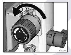
3. Turn ON/OFF switch to ON position.
