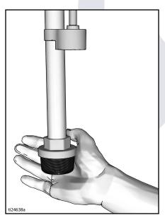
7. Fill throat packing nut with TSL to prevent premature packing wear. Do this daily or each time you spray.
