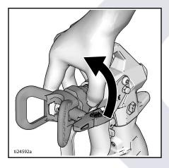
3. Remove fluid intake and drain tube from paint, wipe excess paint off outside.
