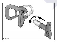
3. Screw assembly onto gun. Tighten.
