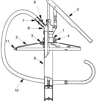
Remove the cover of the lubricant pail and place the dispenser cover on the pail. Lock the cover in place with the three thumbscrews (11). Insert the barrel of the dispenser through the cover and to the bottom of the pail. Tighten the clamp to the barrel.
