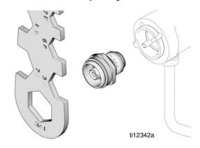
4. Install new diffuser into gun. Torque to 155-165 in-lb (18-19 N•m).
