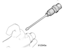
7. Insert air plug nut. Torque to 155-165 in-lb (18-19 N•m).
