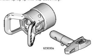
3. Remove diffuser assembly with gun tool.
