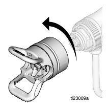
2. Install spray tip into cap assembly.
