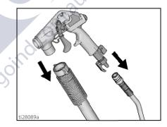
To ensure proper gun function for future use, remove and clean needle components and apply a few drops of light oil to:
