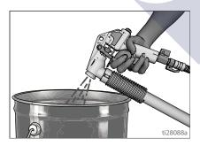
3. Remove nozzle from gun. Trigger gun into bucket until most of texture mix is pumped out. Allow water to flow through gun until gun is clean.
