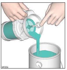
c. Lift up the Strainer and look to verify you can see *crossbars* in the bottom of the Funnel. If not, the cup is overfilled. Pour excess paint back into the paint can.
