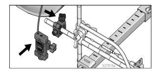
9. Attach light on top of filter cap or on the frame.
