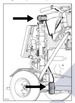
10. Route switch wires down to battery and connect to the (+) and (-) terminals, and route jumper through gun cable hole.
