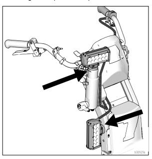
5. Route wires up to the battery and connect to the (+) and (-) terminals.
