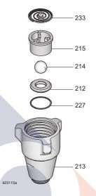
12. Install intake valve on cylinder. If a wrench is used torque as follows:
