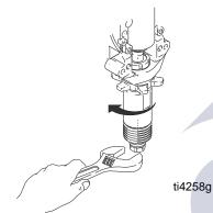
12. Remove pin and piston rod from cylinder.
