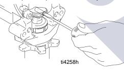
Soak all leather packings in SAE 30W oil for 1 hour minimum prior to assembly. Stack male gland (204). Alternately stack UHMWPE (203) and leather (223) packings (note orientation). Install female gland (224). Install seal (201) and packing nut (202) and o-ring (228).
