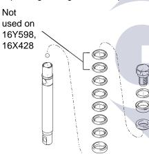
8. Remove throat packings and glands from cylinder. Discard throat packings and glands.
