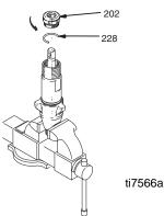
2. Unscrew intake valve from cylinder.
