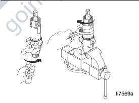
13. Torque packing nut (202) as follows:
