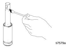
20. Grease o-ring (221) and place on sleeve. Slide sleeve/piston rod assembly into bottom of cylinder. Replace o-ring (207) if desired.
