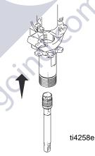
10. Insert piston rod into cylinder with pin hole up and piston valve down. Insert pin into piston rod and crank shaft.
