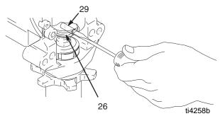
5. Disassemble intake valve. Clean and inspect. O-ring (227) may require a pick for removal.
