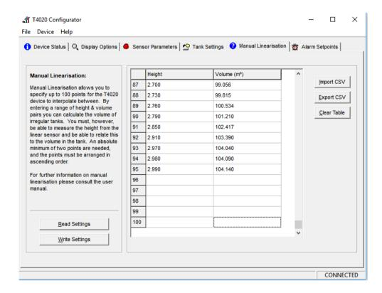
If 96 lines or more are input, the gauge will need to be returned to OLE for a reset and reload of firmware. (this can cause the gauge to display 0 Ltr, or display HIGH)
