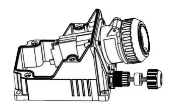
Loosen the cover screws and detach the cover from the wall socket. Open the cable gland and push the cable through it. Strip the cable outer sheath to a suitable length.
