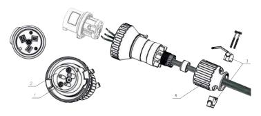
Unscrew the screws (1) near the pins inside the front part (2) until you can detach the front part from the housing.
