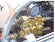
Gearbox drive Pressure gauge Safety valve Brass unloader Thermal dump Brass strainer Bertolini pump
