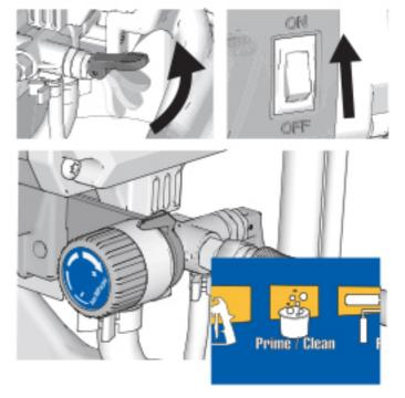
When Pump Armor comes out of drain tube, turn Pressure Control Knob to lowest setting and Power Switch OFF.
