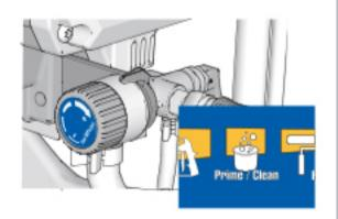
With the trigger lock in locked position, unthread spray tip and guard assembly from gun. Place in waste pail for further cleaning.
