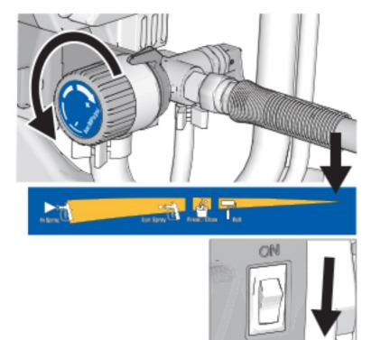
4 Lower Prime/Spray Valve down to SPRAY and install inlet strainer on suction tube for storage.
