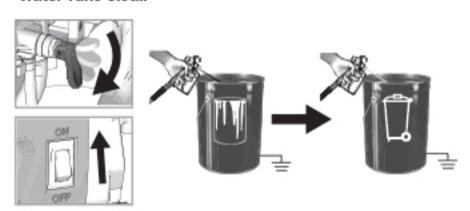
Turn Pressure Control Knob to lowest setting and release trigger. Turn gun trigger lock to locked position. Lift the Prime/Spray Valve up to **PRIME**. Turn Power Switch **OFF**.
