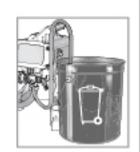
3 Submerge suction tube in water if spraying water-based material or flushing fluid if spraying oil-based.
