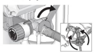
2 Turn gun trigger lock to locked position. Unthread spray tip and guard assembly.
