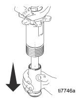
Invert piston rod and sleeve and pound on hard surface until piston rod comes out of sleeve.
