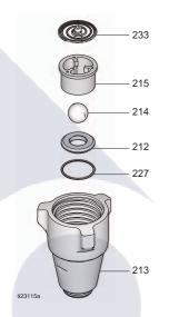
12. Install intake valve on cylinder. If a wrench is used torque as follows:
