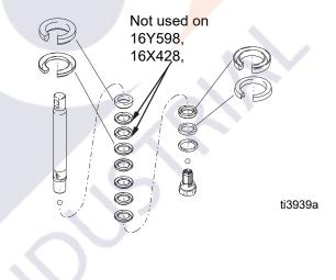
15. Soak all leather packings in SAE 30W oil for one hour minimum prior to assembly. Stack male gland (219) on piston rod. Alternately stack UHMWPE (208)and leather (218) packings (note orientation) on piston rod. Install female gland (217). Install piston wiper (216) and backup washer (229) (note orientation) on piston valve (210). The special sealing patch on piston valve threads is good for four repackings. Use thread sealant on piston valve threads after four repackings.
