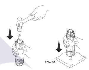
Remove piston rod from sleeve, or remove sleeve from cylinder. Mark IV and Mark VII models: Remove sleeve spacer (230) from sleeve.
