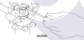
Soak all leather packings in SAE 30W oil for 1 hour minimum prior to assembly. Stack male gland (204). Alternately stack UHMWPE (203) and leather (223) packings (note orientation). Install female gland (224). Install seal (201) and packing nut (202) and o-ring (228).
