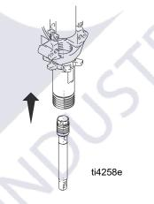
10. Insert piston rod into cylinder with pin hole up and piston valve down. Insert pin into piston rod and crank shaft.
