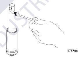
9. Grease o-rings (221) and place on sleeve. Slide sleeve/piston rod assembly into bottom of cylinder. Replace o-ring (207) if desired.
