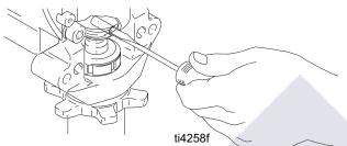
11. Remove piston valve from piston rod with a wrench.
