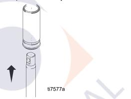
8. Grease top inch or two of piston rod that will go through the cylinder throat packings.
