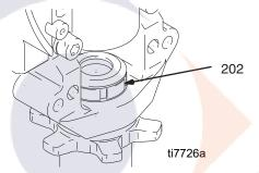
9. Invert piston rod and insert into cylinder to force out throat packings.
