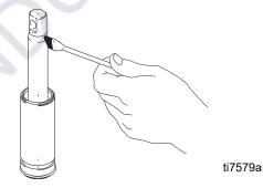
20. Grease o-ring (221) and place on sleeve. Slide sleeve/piston rod assembly into bottom of cylinder. Replace o-ring (207) if desired.
