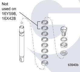
8. Remove throat packings and glands from cylinder. Discard throat packings and glands.
