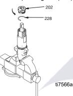
2. Unscrew intake valve from cylinder.
