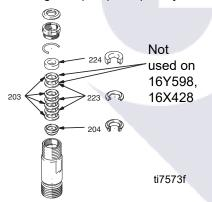
5. Install seal (201) into packing nut (202). Install o-ring (228) onto packing nut. Loosely install packing nut into cylinder.
