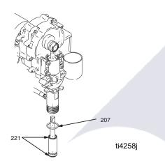
21. Torque seal and packing nut (202) to the following:
