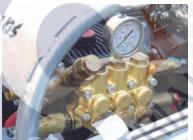
Gearbox drive Pressure gauge Safety valve Brass unloader Thermal dump Brass strainer
