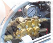
Gearbox drive Pressure gauge Safety valve Brass unloader Thermal dump Brass strainer Bertolini pump
