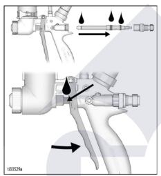
2. **Pressurized hopper gun only:** If lid is too loose and leaks air when pressurized, adjust the four lid clamps to tighten lid.
