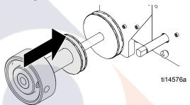
Secure pulley and wheel into place with clamp (engagement wheel pulley will still be able to rotate freely).
