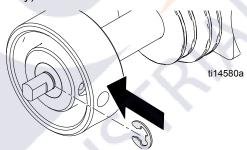
8. Slide pulley onto short axle.
