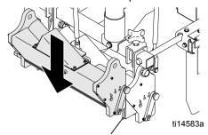
5. Slide single pulley over long axle.
