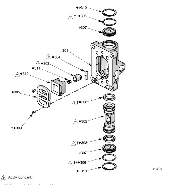
Fig. 15. Pneumatic Valve Assembly
