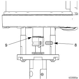
Fig. 12 Retaining spring and connector pin
