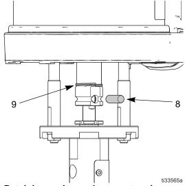
Fig. 3 Retaining spring and connector pin
