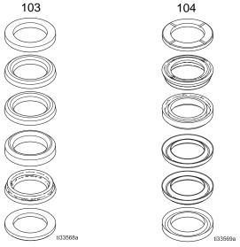
Fig. 7 Packing seal sets
