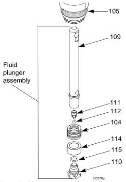
Fig. 6 Fluid plunger assembly
