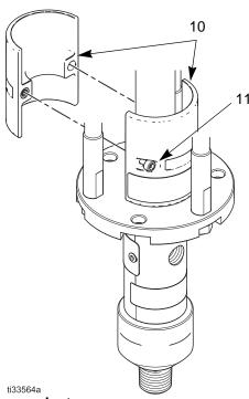
Fig. 2 Remove dust cover
