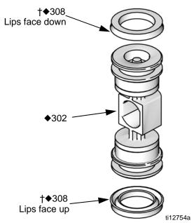
Fig. 16. Pneumatic Valve U-cup Installation
