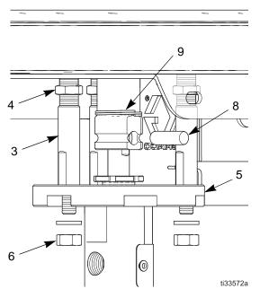
Fig. 18 Retaining spring and connector pin
