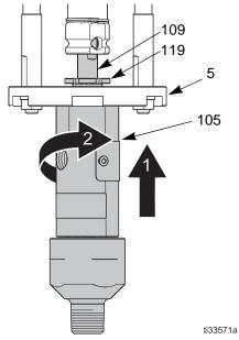
Fig. 11 Reconnect fluid cylinder
