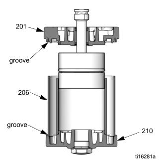
Fig. 21. Align Shield in Grooves on Covers
