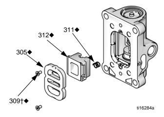
Fig. 14. Pneumatic Plate Removal
