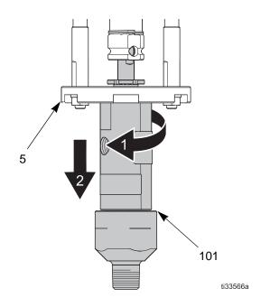
Fig. 4 Remove fluid cylinder
