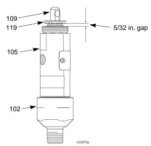
Fig. 9: Tightening the packing nut
