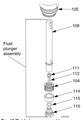
Fig. 10 Fluid plunger assembly
