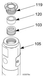
Fig. 8 Top packing seal assembly
