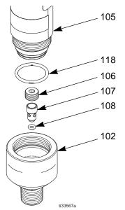
Fig. 5 Fluid cylinder cap assembly
