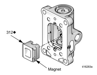
Fig. 17. Pneumatic Valve Cup Installation
