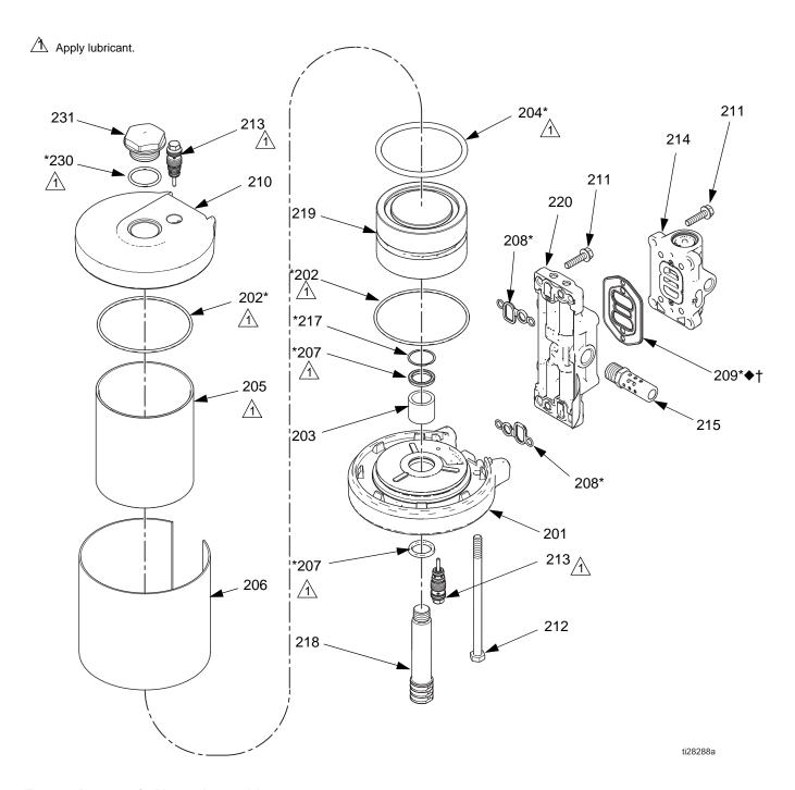
Fig. 20. Pneumatic Motor Assembly
