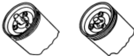
UNLOCKED LUGS PARRALLEL TO SLOT
