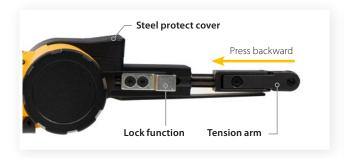
In order to release the belt, press the tension arm towards the steel protect cover to release lock function. Open the protect cover by loosening the cover knob.
