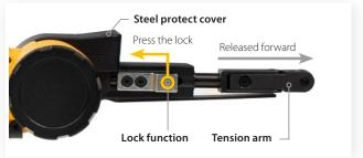
Replace with a new belt. Close the protect cover and tighten the cover knob. Fixate the new belt by pressing the lock towards the steel cover – which releases the tension arm forward.
