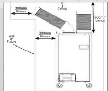
Installation of Extended Hot Exhaust Ducting to Outdoors – (Optional) Hot Exhaust discharge air can be removed from the airconditioned space with flexible duct.
