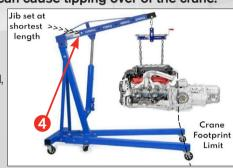
5 Use the jib settings to create a balanced load within the footprint of the crane.
