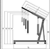
4 Off centre loading and unbalanced loads or loads that mount outside of the crane's footprint can cause tipping over of the crane.
