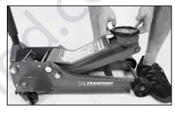
5. Rotate the Pump handle anti-clockwise to the release position and lower the lift arm.
