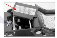
2. Remove the Filler Bung and if required. Refill with \*32 Grade Hydraulic until the oil is approximately 6mm below the filler hole then replace the Filler Bung.
