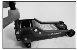
6. Reposition the Pump handle to the horizontal position and turn the Pump handle clockwise back to the raised position.
