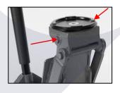
9. The Release mechanism Universal Joint should be cleaned using an aerosol degreaser and after drying should be lubricated with a light bearing grease to ensure long life and prevent premature wear.
