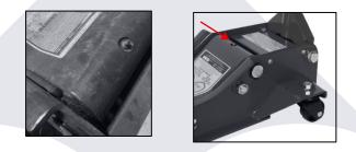
7. All lower lift arm pivots and pins in all linkages should be cleaned using an aerosol degreaser and after drying should be lubricated with a Light Bearing Grease or 30/40W Machine Oil to ensure long life and prevent premature wear.
